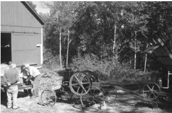
An Attraction Provided by Bill Roberts (white shirt at left) at the Annual Picnic Was a 6 hp 100 yr old Abenague Engine (right), Running an Antique Water Pump Using a Belt Drive. This Engine is the Same Model as Used by Rod and Fred Doolittle's Father on the Doolittle Farm Which Sat at the Bottom of the Hill Below the Visitor Center.
