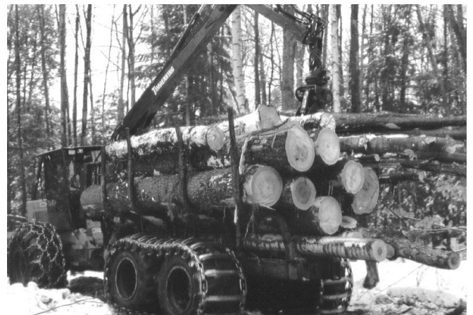
Forwarder Working in the Harvest Area (Trees are being placed in the "bunk")
